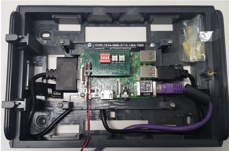
2. Once the ferrite bead is in place, crimp the Ethernet cable at the terminating end.
